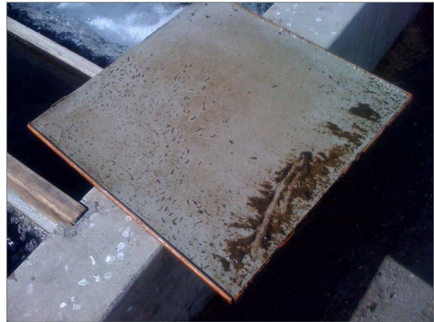
Coated with TruNano Marine Armor, this metal plate was submerged in fresh water for two months. It shows minimal growth, and is easily wiped clean.
